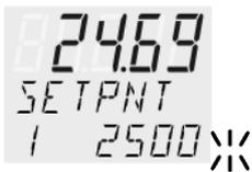
1. By pressing the key
