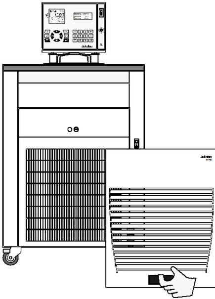
In dusty environments, the refrigerating machine's condenser should be cleaned by vacuuming every 1 to 2 months. The condenser is located behind the venting grid on the front of the unit, which can be taken off by removing the screws.
