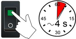
After eliminating the malfunction, turn the mains power switch off and on again to cancel the alarm state.
