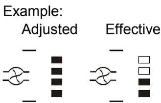
Adjustable pump capacity stage 1 ... 4
