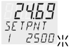
1. By pressing the key
