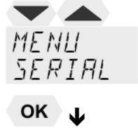
For communication between circulator and a PC or a superordinated process control system the interface parameters of both units must be identical.
