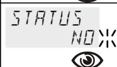
An ATC calibration is to be carried out. Set to >NO<
