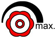
Set the max. permissible feed pressure (example: 2 bar) by slowly closing the adjusting valve (13) on the rear and looking at the manometer (5).
