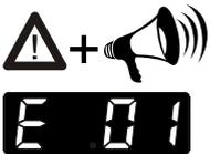
This safety installation is independent of the control circuit. If the low liquid level protection device is triggered, a complete shutdown of the compressor and circulating pump is effected. The alarm is indicated by optical and audible signals (continuous tone) and on the LED-DISPLAY appears the error message "Error 01".
