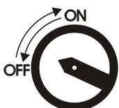
After eliminating the malfunction, press the mains power switch off and on again to cancel the alarm state.
